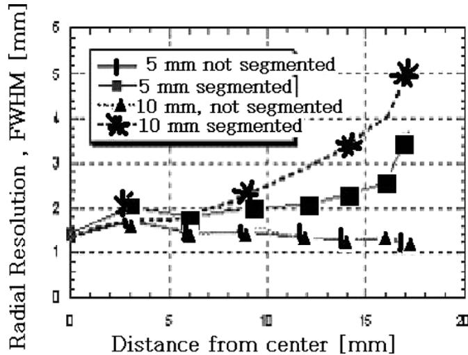
Fig. 9. PSF of a point source as a function of its distance from the center of the FOV for 4 different detector configurations: 1) RatCAP (40 mm ID) and 5 mm LSO crystal length ( $\blacksquare$ ), 2) RatCAP (40 mm ID) and 10 mm LSO crystal length ( $*$ ), 3) tomograph with depth measurement capability (40 mm ID) and 5 mm LSO crystal length ( $+$ ), and 4) with depth measurement capability (40 mm ID) and 10 mm LSO crystal length ( $\blacktriangle$ ).
