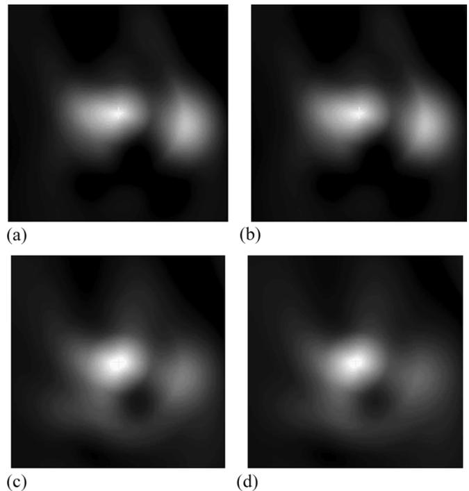
Fig. 8. Image of two point sources. (a) 2-D data mode. (b) 3-D mode with ring difference = 1. (c) 3-D mode with ring difference = 3. (d) 3-D mode with ring difference = 5.
