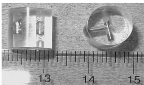
Fig. 3.  $^{68}\text{Ge}$  phantoms of two point sources and an L-shaped source.
