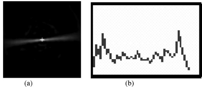
Fig. 5. A line source (a) was generated and its intensity profile (b) at the projection perpendicular to the line source was used for normalization.
