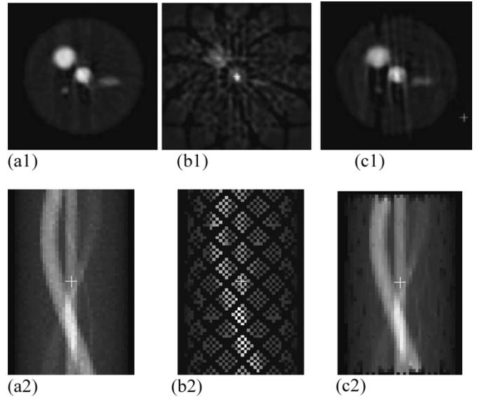
Fig. 10. (a1) Reconstructed image from a fully sampled sinogram (a2). (b1) Reconstructed image from a realistic RatCAP geometry sinogram (b2). (c1) Reconstructed image from interpolated sinogram (c2).
