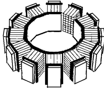
Fig. 1. First prototype of RatCAP consisting of  $12 \times 4 \times 8$  arrays of LSO+APD detector blocks.
