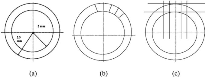
Fig. 6. Simulation geometries. (a) Cylindrical PET. (b) Discretized PET with no gaps. (c) Discretized PET with gaps between blocks (block detector geometry).
