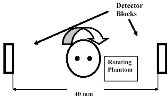
Fig. 2. Phantoms were placed on a rotational platform and rotated in  $\sim 13$  steps through 180 degrees.
