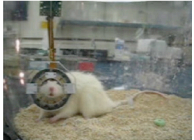
Fig. 5. Awake rat wearing the RatCAP that is supported by the tether and mechanical counterbalance system.
